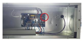
4. Check the fuse (Qualified personnel only. Only carry out when there is no current. Non-qualified personnel please contact Delta-Temp). To do this, remove the cover on the back of the device with 8 screws.
