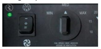
1. Check whether the LED light on the control panel glows green. Red light means error.
