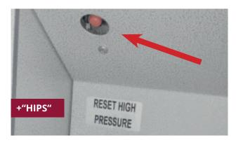
9. **Error message +"HIPS"**. After doing these checks and fixing the problem, press the "Reset" button.
