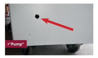
7. Error message +"Pump". Unplug the air conditioner and check if the pump can move freely. Insert a long flathead screwdriver into the hole on the left side of the unit and attempt to rotate the pump. If the pump does not rotate, there is a defect: contact Delta Temp.
